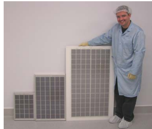
10W and 40W SLIVER modules sit beside the new 70W prototype module at the Regency Park plant.
